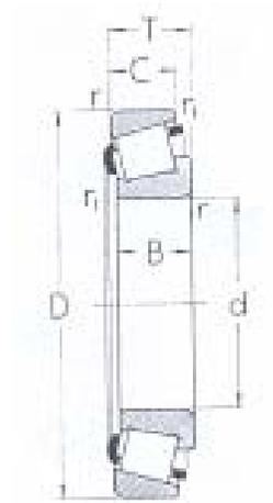
A taper roller bearing and its nomenclature are shown in Fig.14.2.6 above. It is generally used for simultaneous heavy radial load and heavy axial load.
