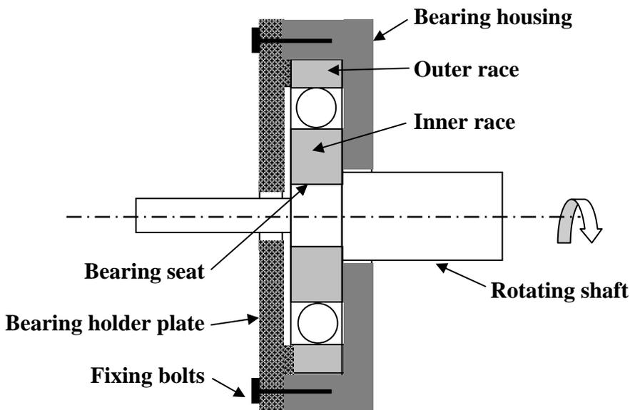
**Fig. 14.2.2** A typical arrangement for housing a bearing
